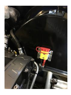
New location on inner wheel arch sufficiently distant from exhaust heat and protected from water spray from road.
