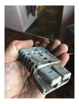
Anderson connector as removed from a 2001 Tuscan. Heavy corrosion on both terminals and casing disintegration. Danger of short circuit leading to electrical fire and/or moisture causing battery to discharge.
